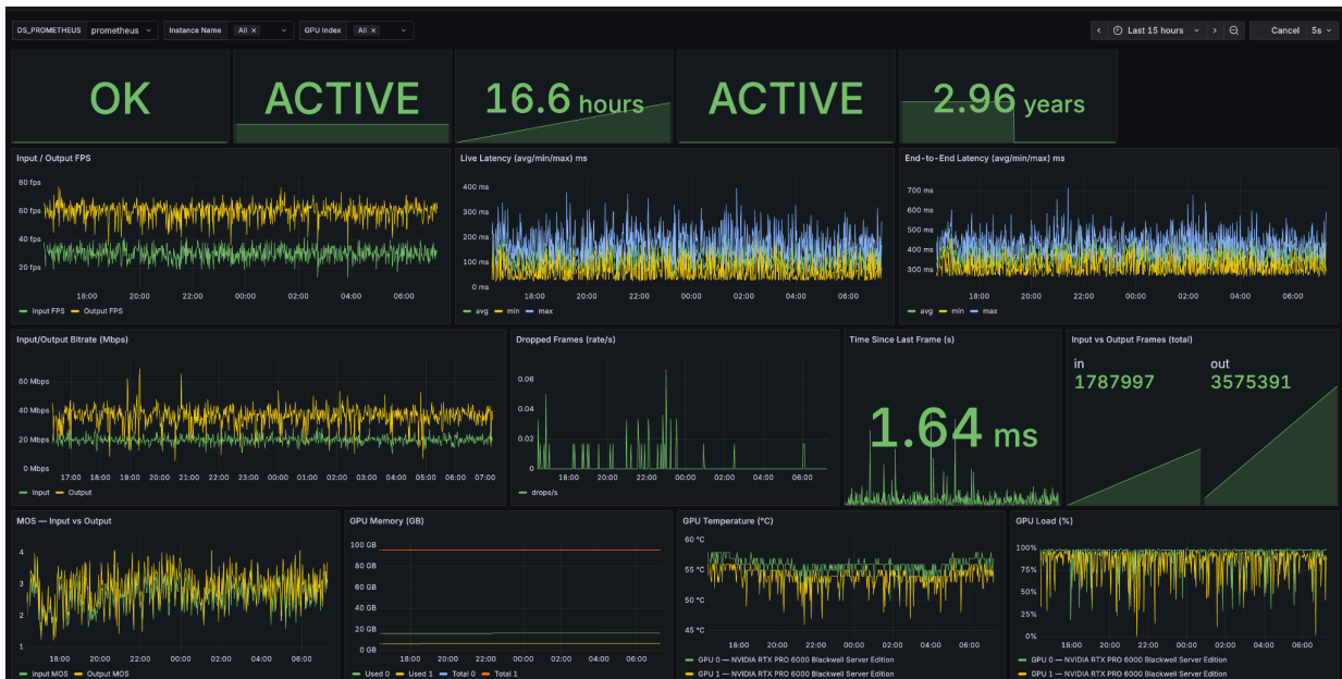
Figure 3 — A Grafana dashboard based on data from the Prometheus metrics endpoint
